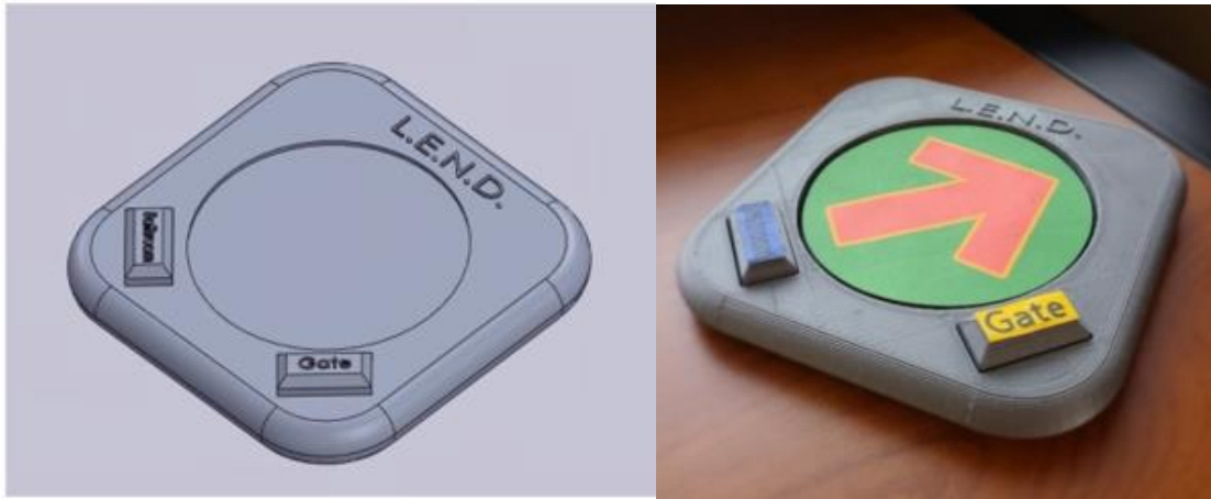
Figure 6: Final Prototype C.A.D. Model in SolidWorks and 3D printed device
